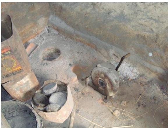
Fig 2 : Melting Pit Furnace ("Bhatta")
