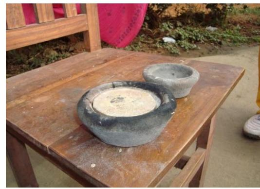
Fig 5: Metal block in the Mould
