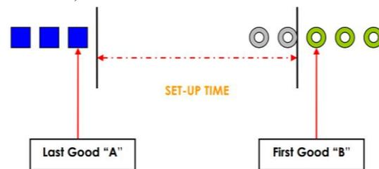
Fig 2. Set up time
