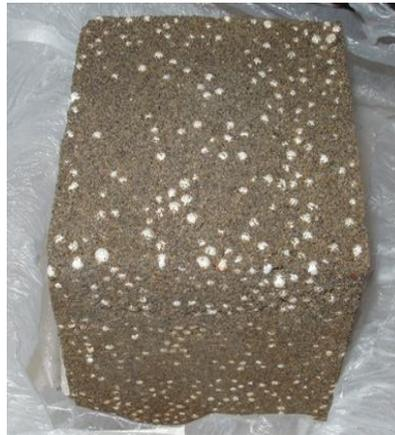
Fig 1: Lightweight fill with EPS beads
