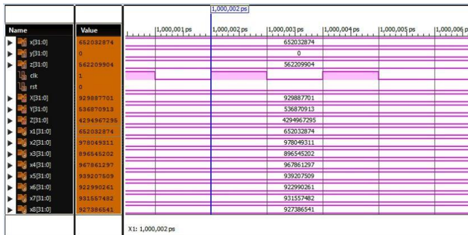
Fig.5: Simulation result that calculate cosine and sine for angle 30° for 32 bit word length.
