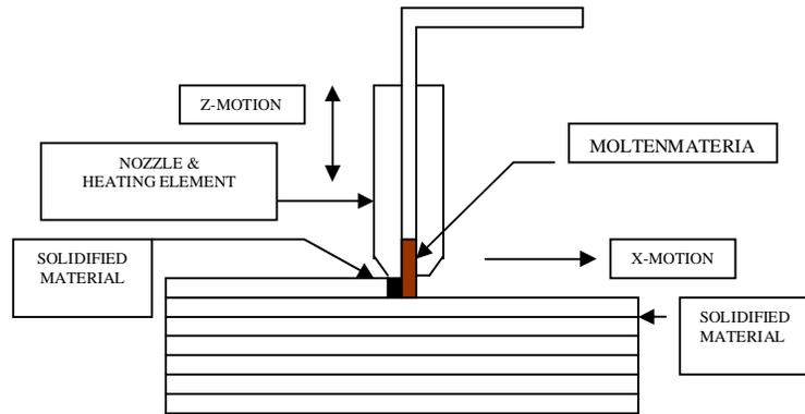
Fig. 1 Fused Deposition Modelling Process
