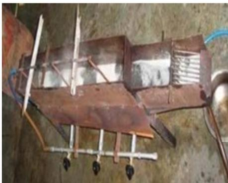
**Figure 15.** Rasogolla cooker developed at IIT Kharagpur for cooking rasogolla under atmospheric pressure.
