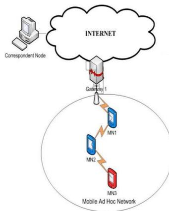
Fig. 1. Architecture of a Hybrid MANET [6]
