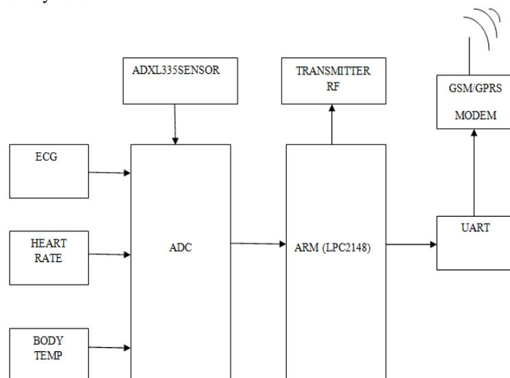
Fig.1. Block Diagram for proposed system
