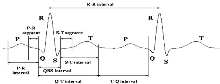
Fig.7. ECG waveform
