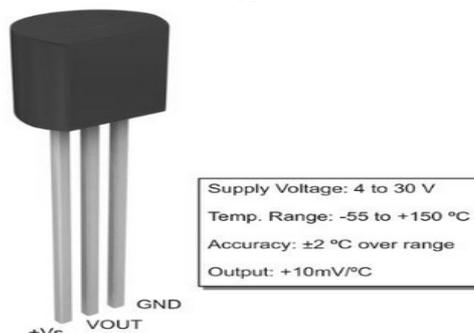
Fig.3. Pin Details of LM35 Temperature sensor
