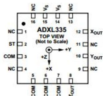
Fig.4. ADXL 335 Pin Configuration.
