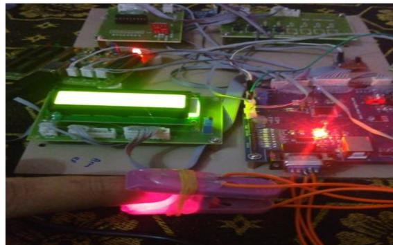
The GSM (Global System for Mobile communication) modem transmits these events to the mobile phones of care takers/ relatives of the fallen human as a message shown as yellow box. This alert message helps to provide immediate assistance and treatment. Temperature, heart rate is displayed in the below output window.
