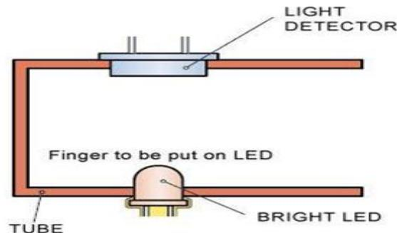
Fig.5. Sensor Construction.
