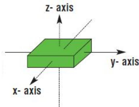
Fig.3. Three-axis direction of MEMS accelerometer
