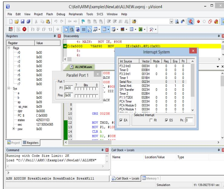
Fig. 9: Output of Keil simulator shown above indicates that though the warning is given to the viewer, instead of moving away he/she is still standing near the television, then first alarm goes off, and finally the television is switched off after approximately 2 minutes i.e. 120 seconds (Pin 4=TV, Pin 1=Alarm).
