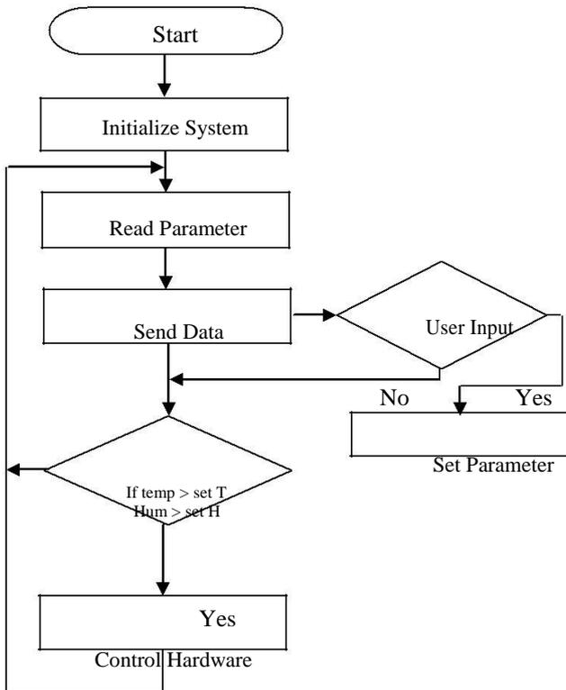
Fig. 3 Flow chart for transmitting station of grain storage system
