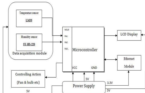
Fig. 2 Architecture of grain storage system
