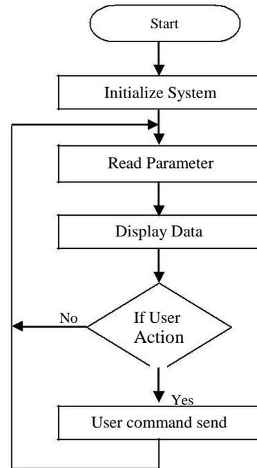
Fig. 4 Flow chart for receiving station of grain storage system
