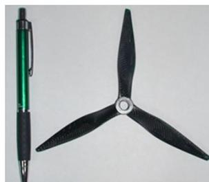
Fig. 2. Three bladed 6"x5"CFRP propellers
