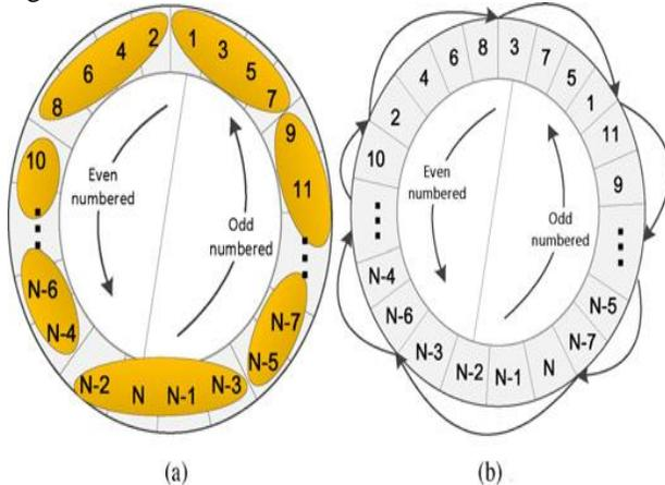
Fig. 2. Frequency interleaved ordering (FIO) with pseudo-random interleaving
