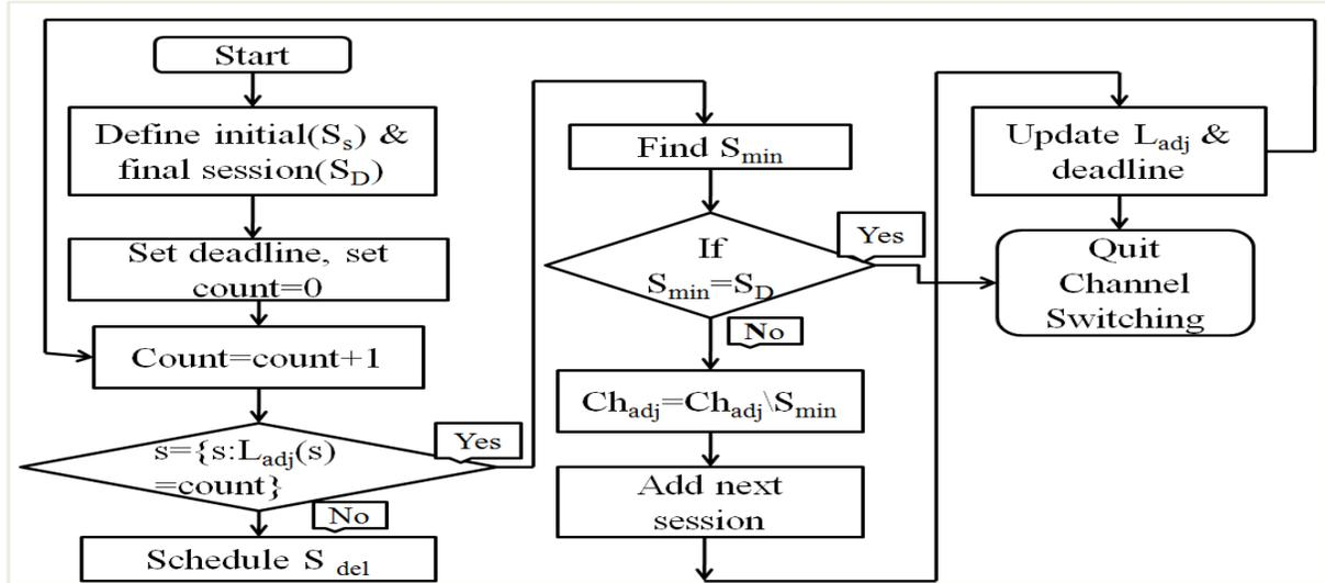
Fig. 4. Channel Switching Mechanism
