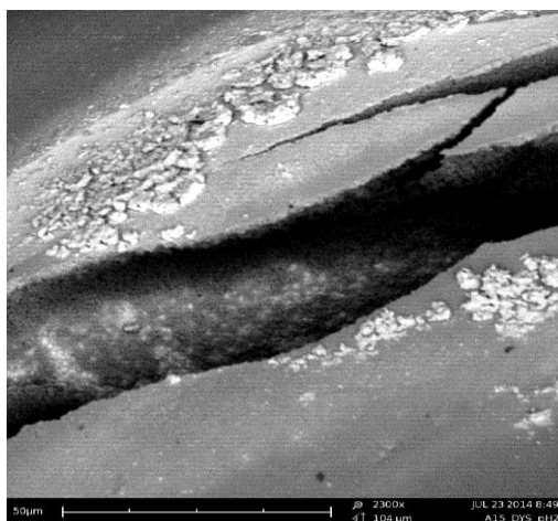
Fig. 9. Polystyrene/amine resin showing breakage and interior loading.
