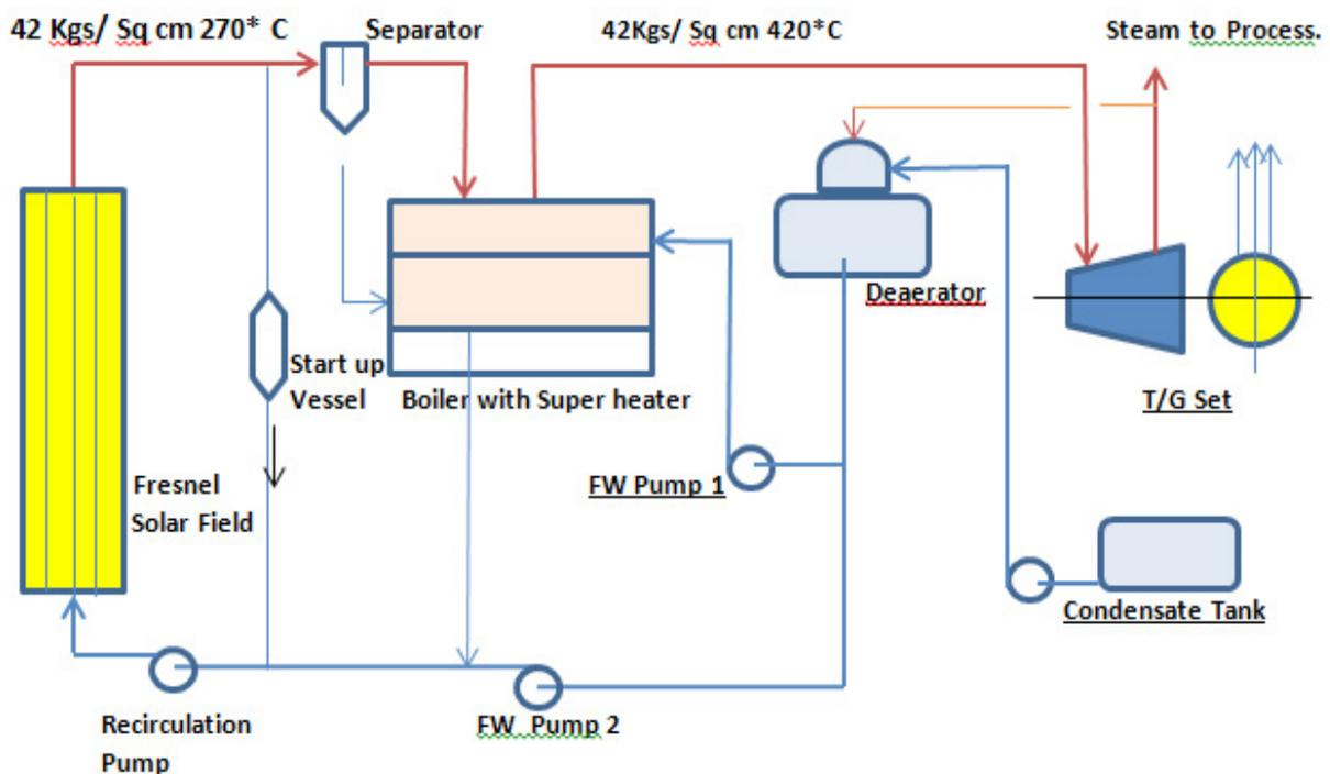
Figure 12. Hybrid solar- bio/fossil fuel steam and electricity generation.
