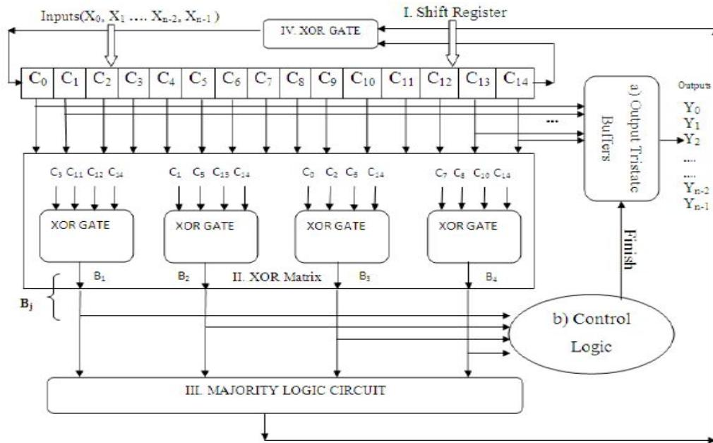
Fig:3.Schematic of the proposed MLDD for 15 bit code word. a) Control logic b) Output tristate buffers
