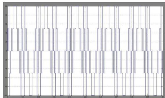
Fig. 4 Output waveform of five level CMLT using SHE Technique
