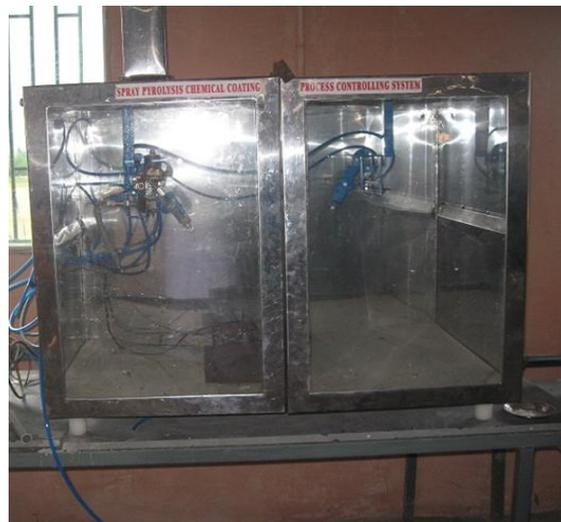
Spray Pyrolysis Chemical Coating Process
