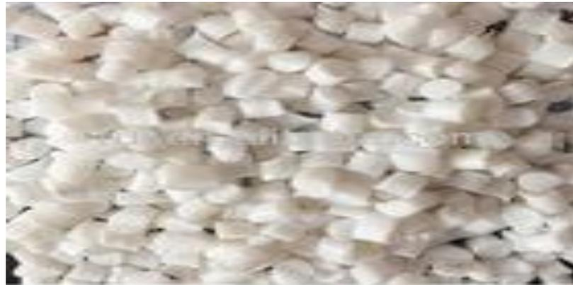
**Fig.1 Thermoplastic starch based resin 11C**
