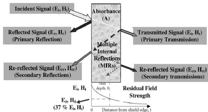
Figure 1. Graphical representation of EMI shielding. (Choudhary.V.et.al., Ref [8] cited in the below list)
