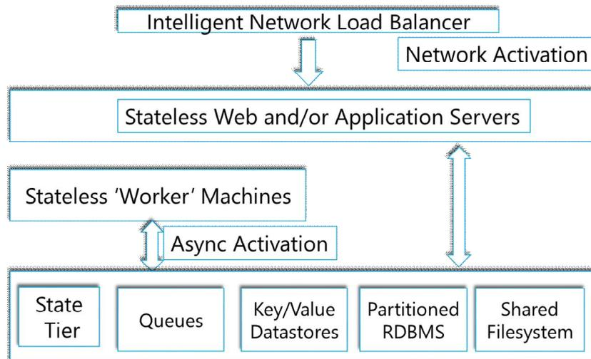
Fig. 15 Inbound Connectivity with Load Balancer
