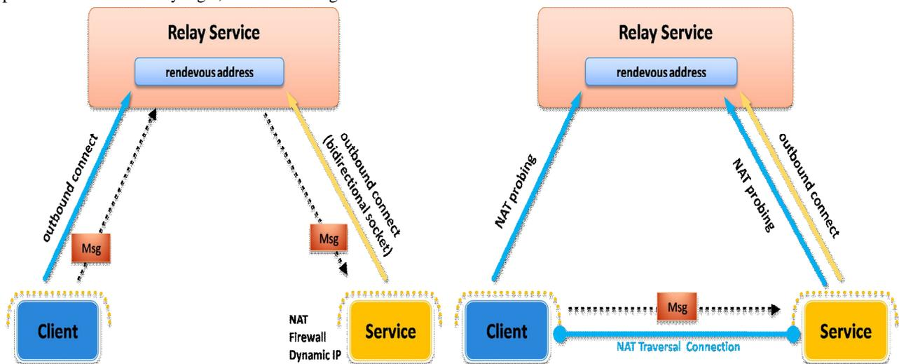
Fig. 13 Establishing a Relay Connection
