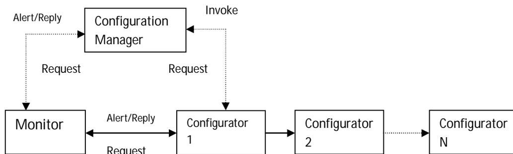
Fig. 4: Chain-of-Configurator-modules architectural style
