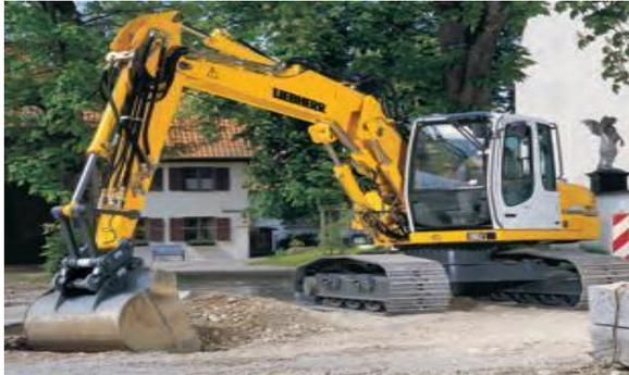
Figure 1 Hydraulic excavator.
