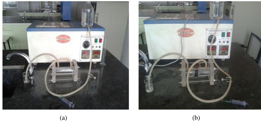
Fig.1 Experimental arrangement of reactors (a) reactor without packed media (b) reactor with packed media
