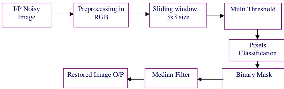
Fig.2: Block Diagram of proposed method
