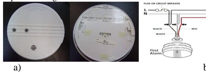
Figure 6. a) Kidde's ionization smoke alarm. b) Diagram of the smoke detector.
