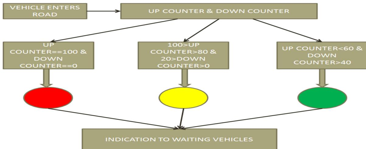
Fig. 2 Flow chart for diversion of vehicles based on traffic density
