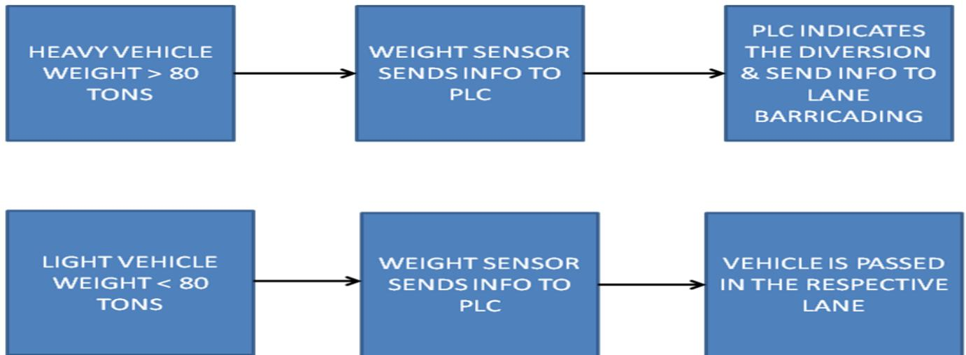
Fig. 1 Flow chart for diversion of vehicles based on weight
