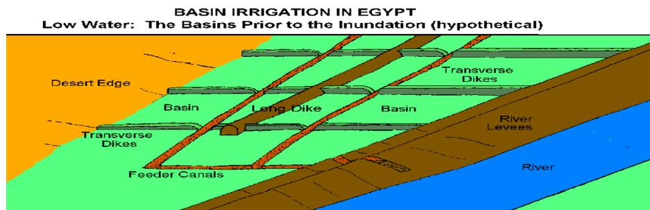
Fig.23. Immersion Irrigation framework
