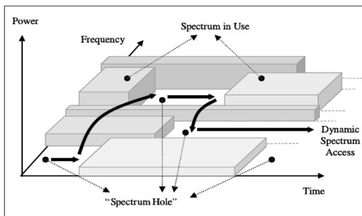
Fig.1 Concept of spectrum hole.
