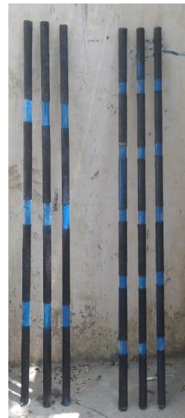
Fig. 3 CFRP wrapped specimens
