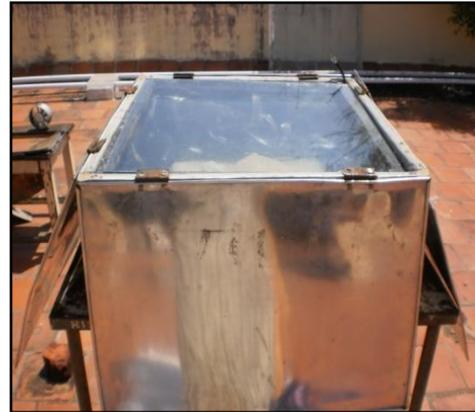
Fig 12: Wax melting chamber
