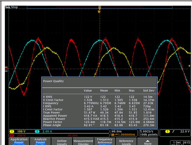
Fig. 14. Experimentally measured RF power coupled by antenna to plasma chamber using Oscilloscope power analyzer, antenna voltage 100 V/div., current through it 2 A/div. and power 200 W/div.
