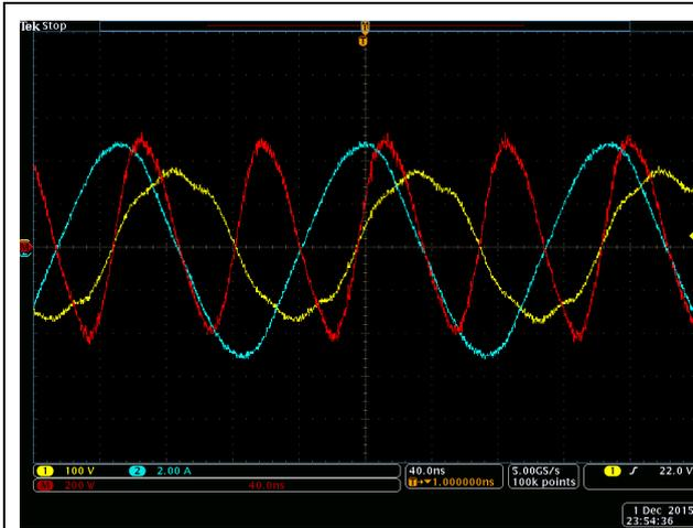
Fig. 13. Experimentally recorded RF antenna voltage 100V/div. and current through 2A/div.
