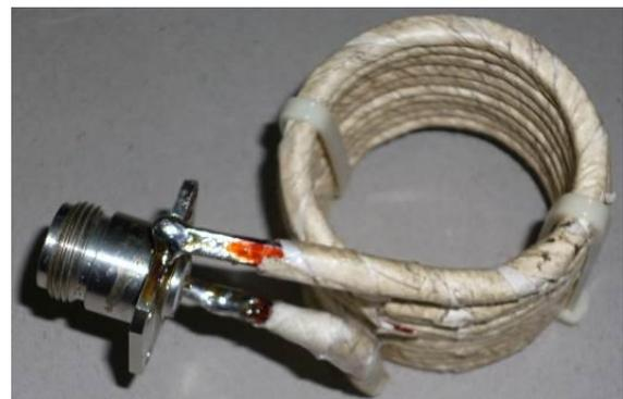
Fig. 1(a). RF antenna made of 4 mm diameter round conductor with 10 turn.
