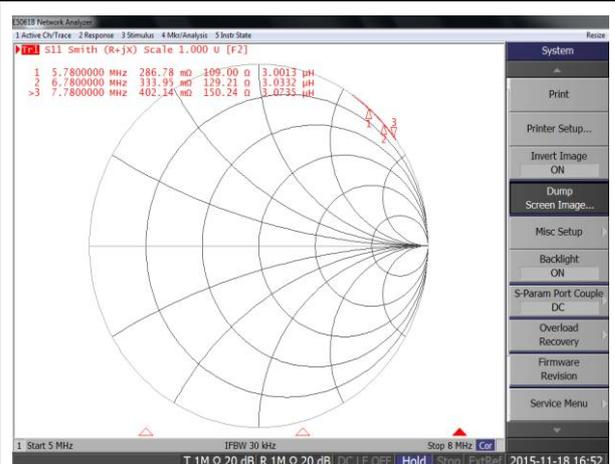
Fig. 2(a). Experimentally measured Smith chart and parameters of RF antenna made of 4 mm diameter round conductor with 10 turn, using VNA.
