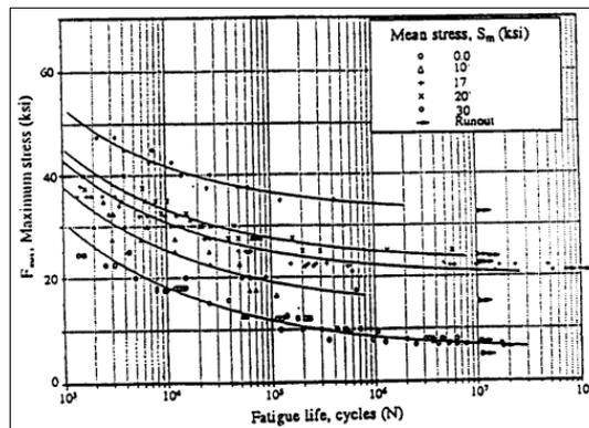
Fig. 4. Stress vs. life to failure in metals.
