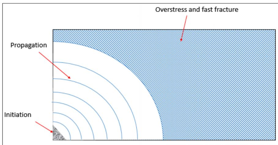
Fig. 1. Fatigue failure in metals.
