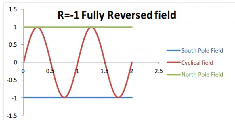
Fig. 3. Bi pole fatigue cycling.
