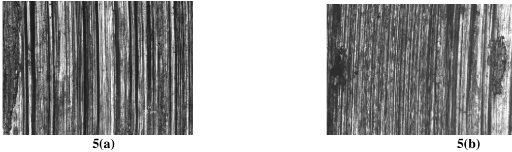
Plate 5: Optical micrographs of worn surfaces of As-cast A356 5(a) and Grain refined and modified A356 ( A_{GRM} ) 5(b)
