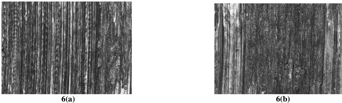
Plate 6: Optical micrographs of worn surfaces of Heat Treated A356 and Grain refined and modified ( A_{GRM-H} )
