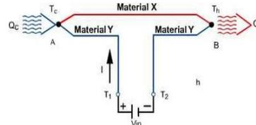
Fig.4 Process on peltier effect
