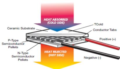
Fig.2 Complete Thermoelectric Module
