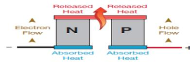
Fig.3 Semiconductors electrically in series and thermally in parallel
