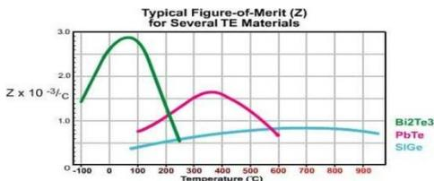
Fig.1 Relative performance or figure-of-merit of various materials
