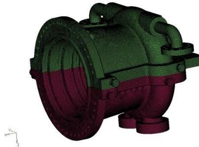
Fig 3: Steam Casing (HP) Meshed Model
