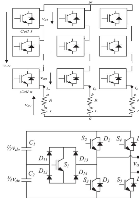
Fig. 4. TCHB: (a) general configuration of the proposed three-phase cascaded multilevel inverter and (b) topology of five-level transistor-clamped H-bridge for each cell.
