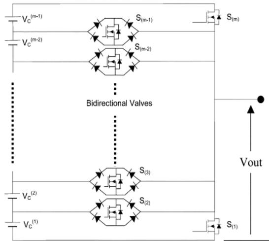
Fig. 1. The m-level transistor-clamped inverter.
