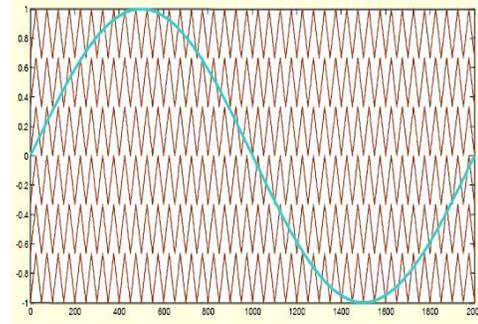
Fig .6. phase disposition PWM.
