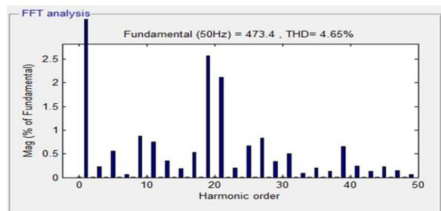
Fig .10. Line voltage harmonics with its THD value of a proposed inverter.
