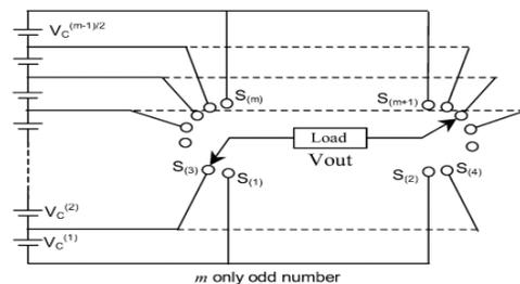
Fig. 3. The m-level inverter using an "H" bridge.
