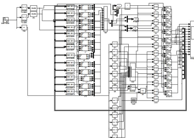
Fig. 5. PWM signal generation with multicarrier phase-disposition modulation.
