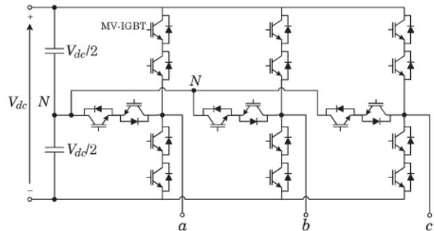
Fig. 2. Three- phase three-level TCC.
