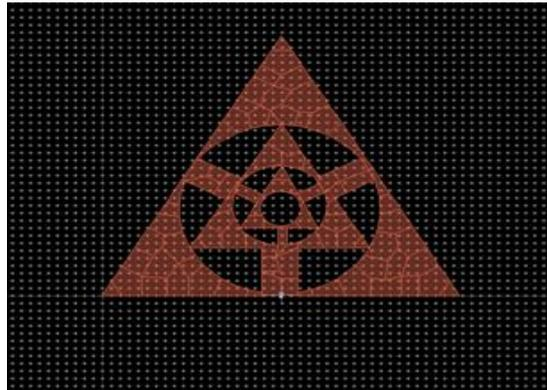
Fig.1. Triangular and circular antenna with coupling patches
