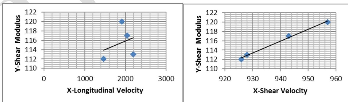
**Fig.10.**Correlation between Longitudinal velocity and Shear Modulus, correlation between Transverse velocity and Shear Modulus
