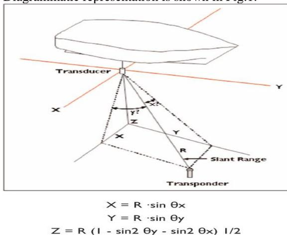
Fig 1. Functioning of USBL System
