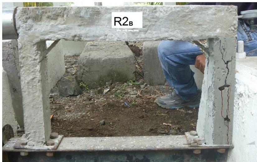
Figure7. Photograph of Corner Braced R.C. Frame R2<sub>B</sub>
