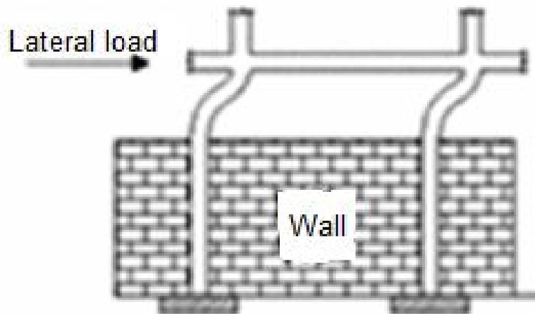
Figure1. Partially infilled frames subjected to Lateral load
