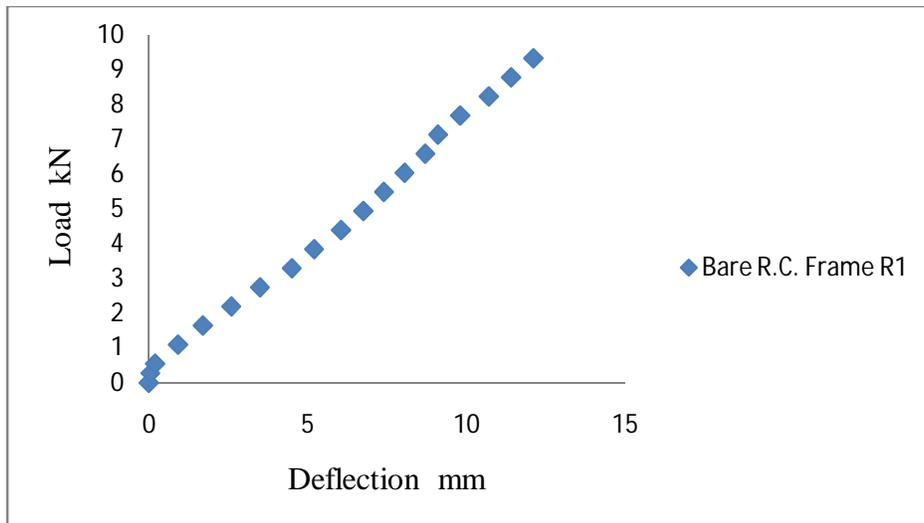
Figure3. Effect of Load over Deflection for Bare R.C. Frame
