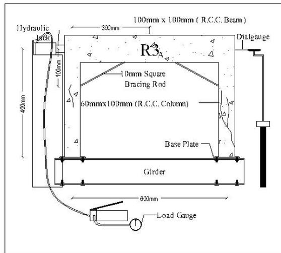
Figure6. Crack pattern for central braced frame R3<sub>A</sub>
