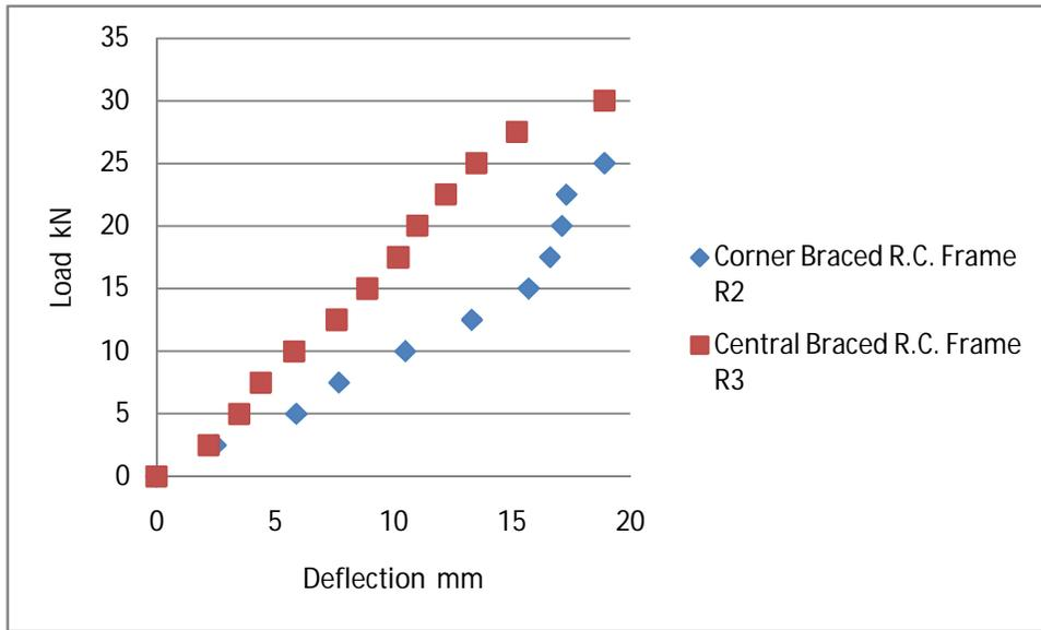
Figure4. Effect of Load over Deflection for Braced R.C. Frames
