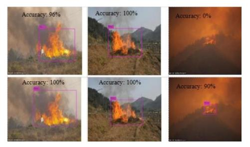
Figure 10. Picture comparison for PCA with YOLOv3 (below) and YOLOv3 (observe). You can observe that PCA with YOLOv3 shows the better location and detection accuracy. The combination method can observe the early fire.
