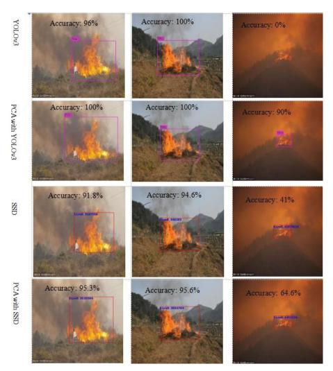
Figure 15. Four methods of image comparison. From the images comparison, you can see that the combination has better location and detection accuracy.
