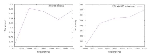
Figure 12. Testing accuracy for SSD (left) and PCA with SSD (right). PCA with SSD shows higher test accuracy. After 50000 iteration times, the test accuracy of PCA with SSD reaches 88. Compared with the combination method, SSD has a little lower test accuracy, 87.6. Here test accuracy means mAP.
