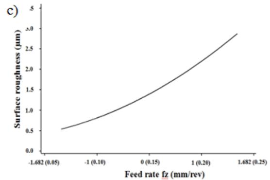
Fig 2 Main Effect of Parameters a) Tool Nose Radius b) Cutting Speed c) Feed Rate
