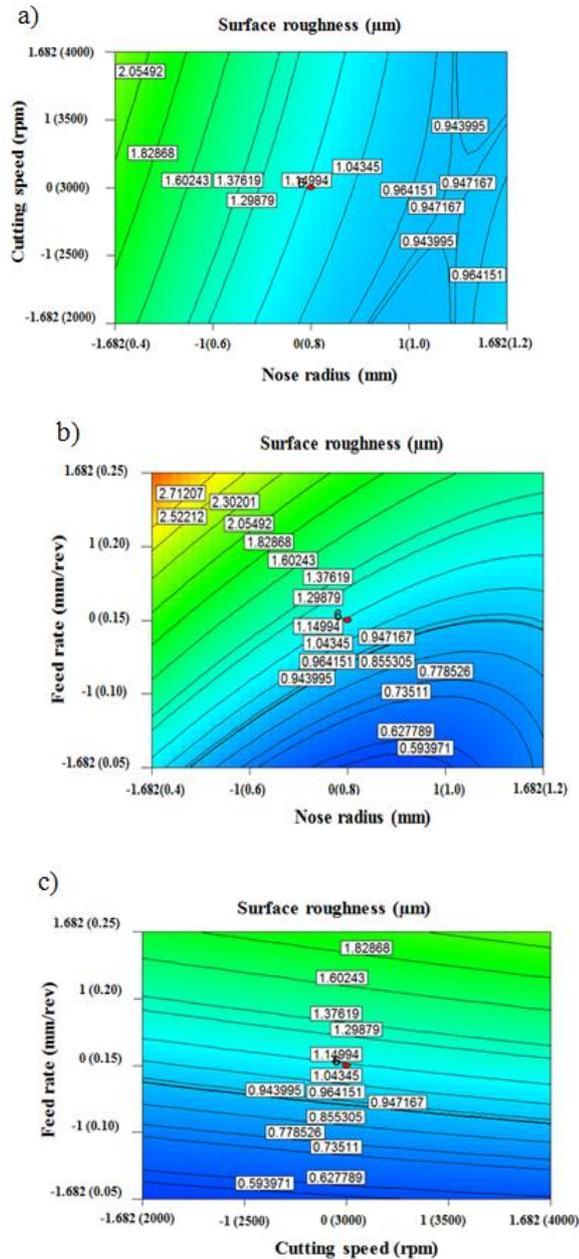
Fig 3 Interaction Effects of input Parameters a) Nose Radius and Cutting Speed b) Nose Radius and Feed Rate c) Cutting Speed and Feed Rate
