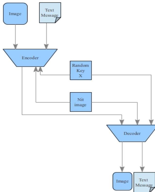
Fig. 3.2 Nit Process entire flow
