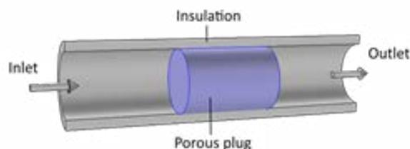
**Figure 1.** Diagrammatic representation of Joule-Thomson impact.
