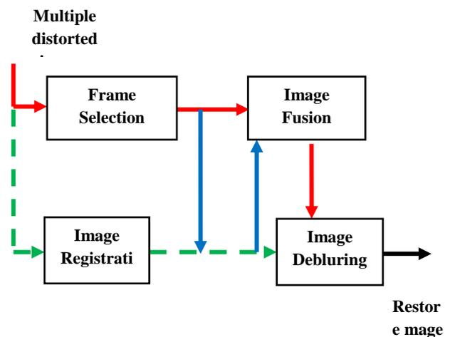
Fig. 1 Block diagram of image restoration for atmospheric
