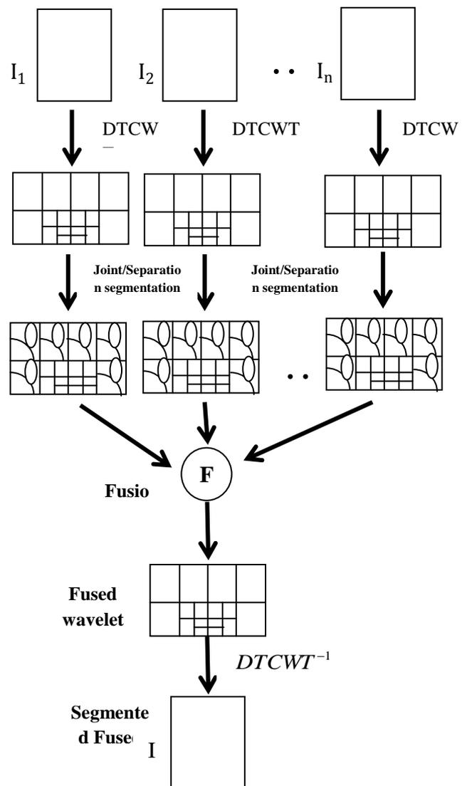
Fig. 3 The Region-based Image Fusion using DTCWT
