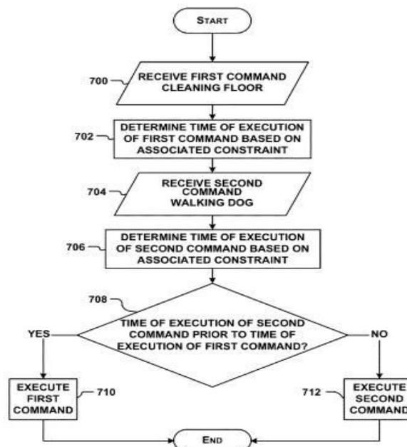
Figure 4 Flow Charts for robotic unit
