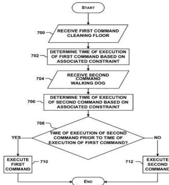
Figure 4 Flow Charts for robotic unit
