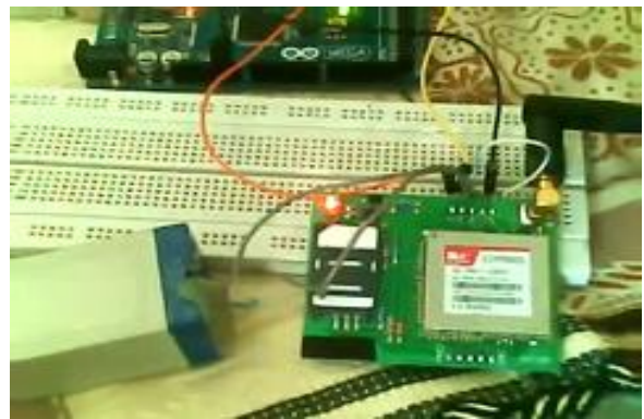
Fig 6 GSM connected with Arduino
