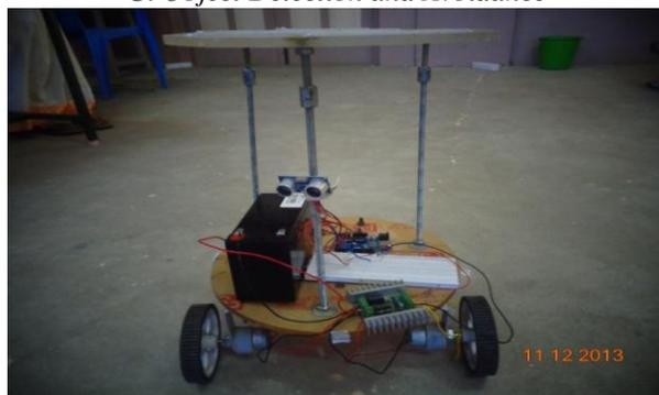
Fig. 7 Object detection and avoidance by using Ultrasonic sensor
