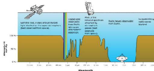
Rough plot of Earth's atmospheric transmittance (or opacity) to various wavelengths of electromagnetic radiation. Microwaves are strongly absorbed at wavelengths shorter than about 1.5 cm (above 20 GHz) by water and other molecules in the air.
