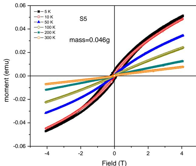
**Fig 3:** M-H curves of ZnO-BiFeO<sub>3</sub> at 300 and 5K
